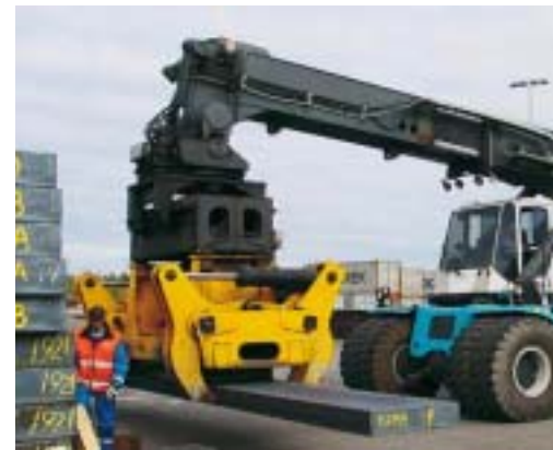
Lift unit for steel slabs and coils.
