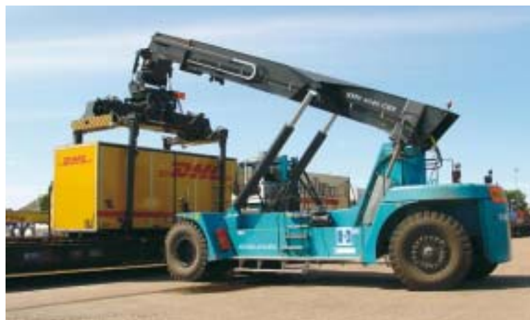
A large Rail Stacker provides extra lifting capacity to load on track 1 or track 2. Trucks with long wheelbase lifts with higher capacity and have longer reach.
